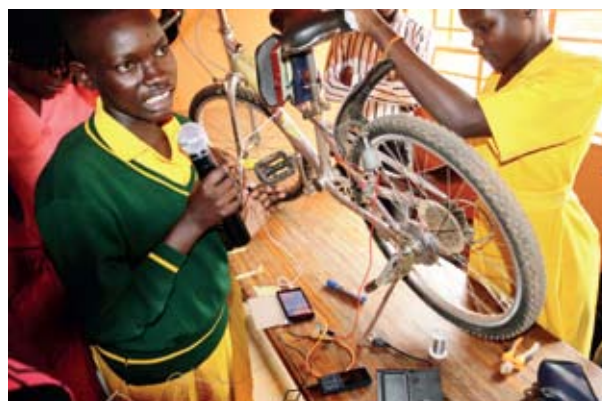
A Student demonstrating how the Bicycle Power Charging System Works during the FAWE Uganda National Science and Innovation Competitions. The Innovation is used to charge phones in rural communities in Northern Uganda.
